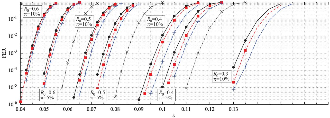
Fig. 3. FER over the BSC with crossover a probability  $\varepsilon$  for several LDPC codes with coding rates  $R_0 = 0.3$ ,  $R_0 = 0.4$ ,  $R_0 = 0.5$  and  $R_0 = 0.6$ , and two different proportions of punctured symbols,  $\pi = 5\%$  and  $\pi = 10\%$ .
