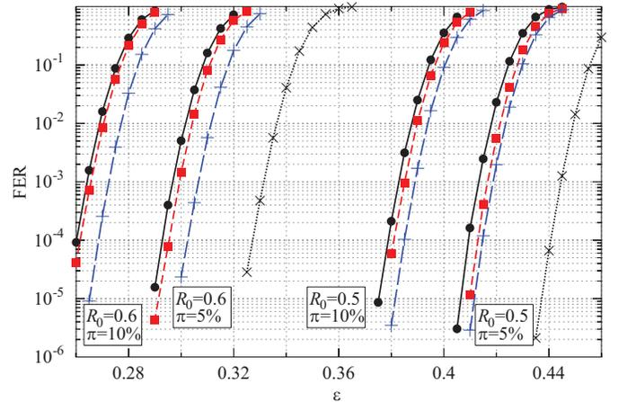
Fig. 2. FER over the BEC with crossover probability  $\epsilon$  for different intentional puncturing strategies. Two LDPC codes with coding rates  $R_0 = 0.5$  and  $R_0 = 0.6$ , and two different proportions of punctured symbols,  $\pi = 5\%$  and  $\pi = 10\%$  were used. See inset in Fig. 1 for symbols and line-styles.
