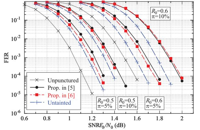
Fig. 1. FER over the AWGN as a function of the signal-to-noise ratio (SNR). Two LDPC codes with coding rates  $R_0 = 0.5$  and  $R_0 = 0.6$ , and two different proportions of punctured symbols,  $\pi = 5\%$  and  $\pi = 10\%$  were used.
